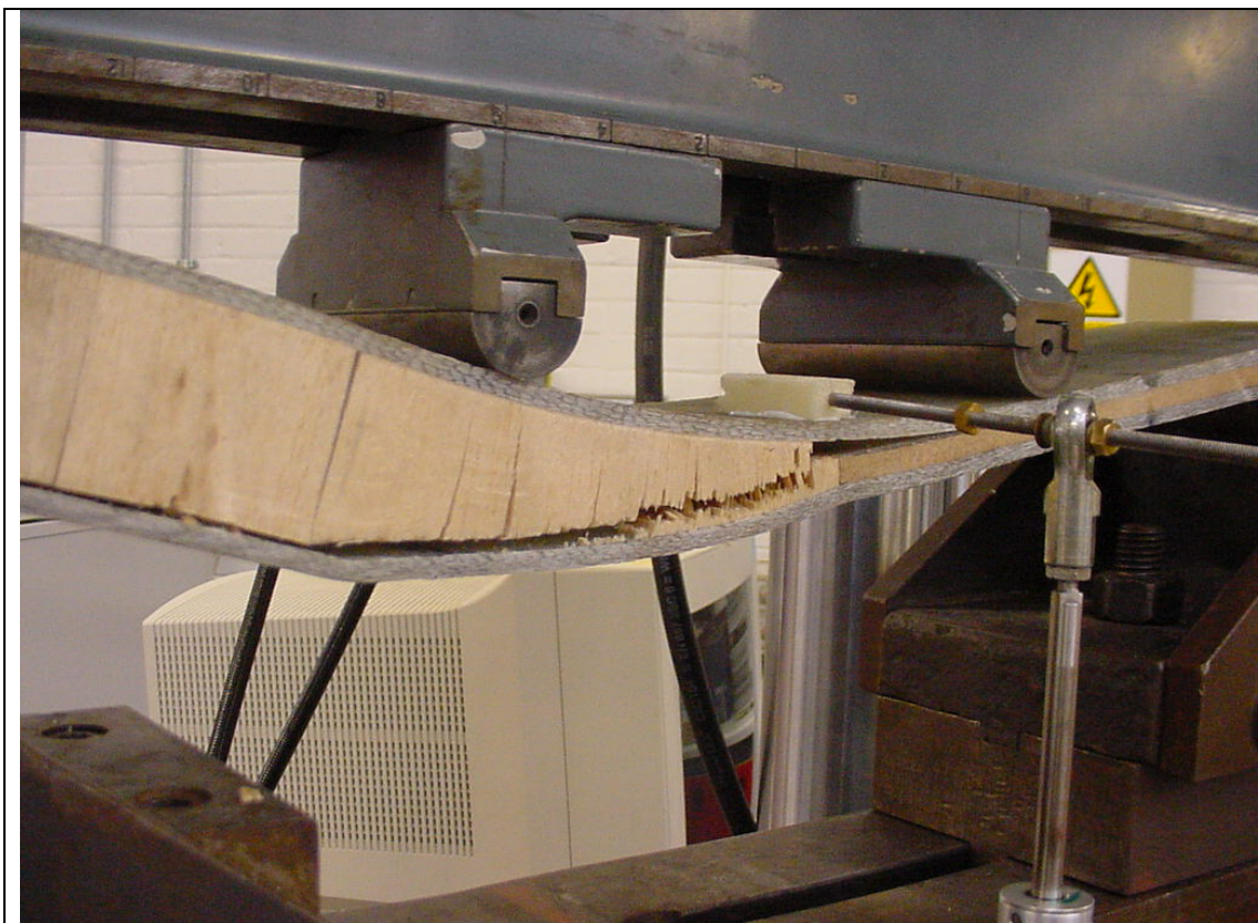
Figure 6.27 Failure of HSC joint in 4-point bending
