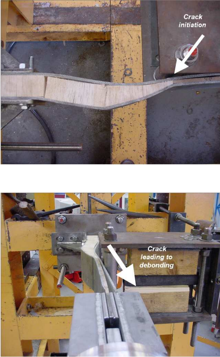
Figure 7.7: Hybrid joint specimen under static compression test (Boyd et.al., 2004)
