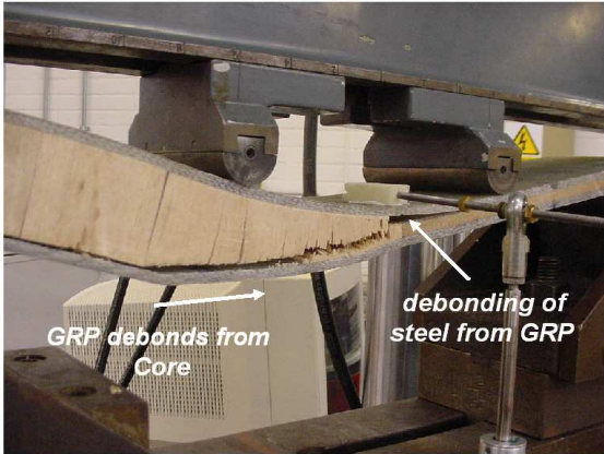
Figure 7.12: Hybrid joint specimen under 4-pt bending test (Boyd et.al., 2004)
