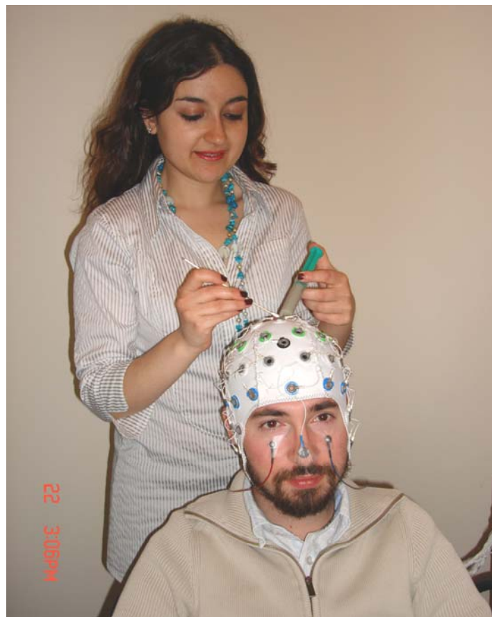
Figure 4-6. Recording of the EEG: A 66-channel EEG cap with Ag/AgCl electrodes; a high chloride, abrasive electrolyte gel is inserted in each electrode location to achieve a DC-stable skin-gel contact for stable operation of the electrodes. Electrodes attached below the eyes for recording of the EOG.
