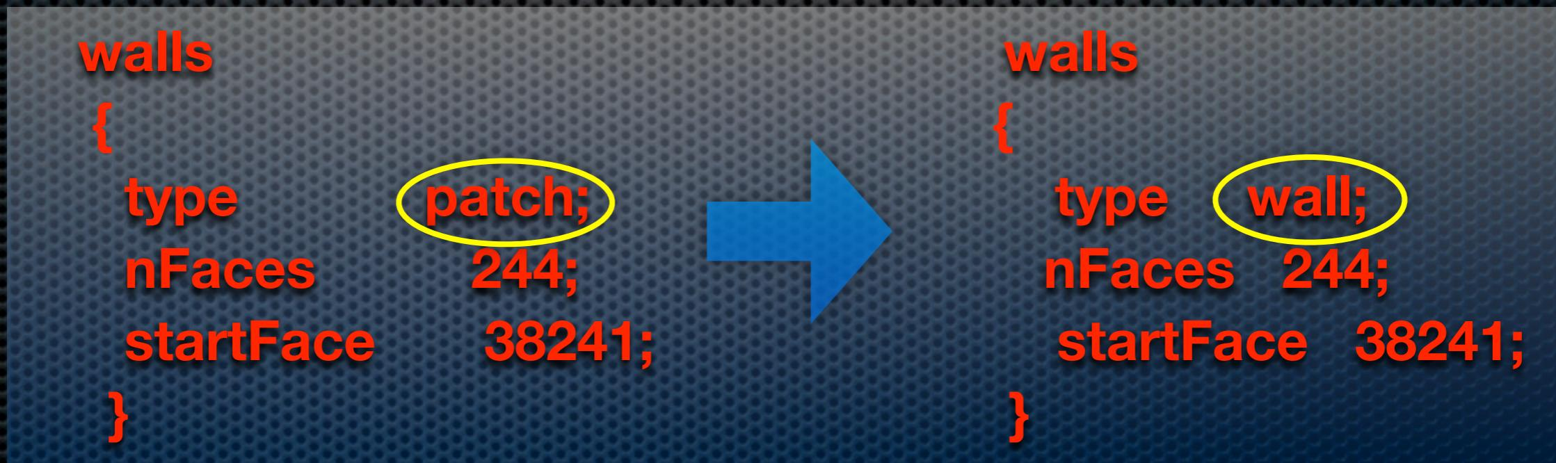
The diagram illustrates the modification of a mesh entry. On the left, a code snippet shows a 'walls' section with a 'patch' entry. The word 'patch' is highlighted with a yellow oval. An arrow points to the right, indicating the transformation. On the right, the code is shown again, but the 'patch' entry has been replaced by a 'wall' entry, also highlighted with a yellow oval.
