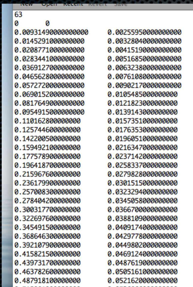
A screenshot of a text editor window showing the content of the 'airfoil.data' file. The window has a menu bar with 'File', 'Open', 'Recent', 'Revert', and 'Save'. The main text area contains a list of coordinates for a 2D airfoil, starting with '63' and followed by pairs of x and y values. The values are floating-point numbers with many decimal places, representing the airfoil's profile.
