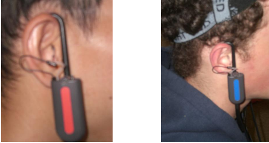
Figure 11: Probe tube in-situ. Left image shows the right REM housing on right ear for measuring the 0° loudspeaker-to-client azimuth conditions whilst right image shows the left REM housing on the right ear for measuring the 45° loudspeaker-to-client azimuth conditions.
