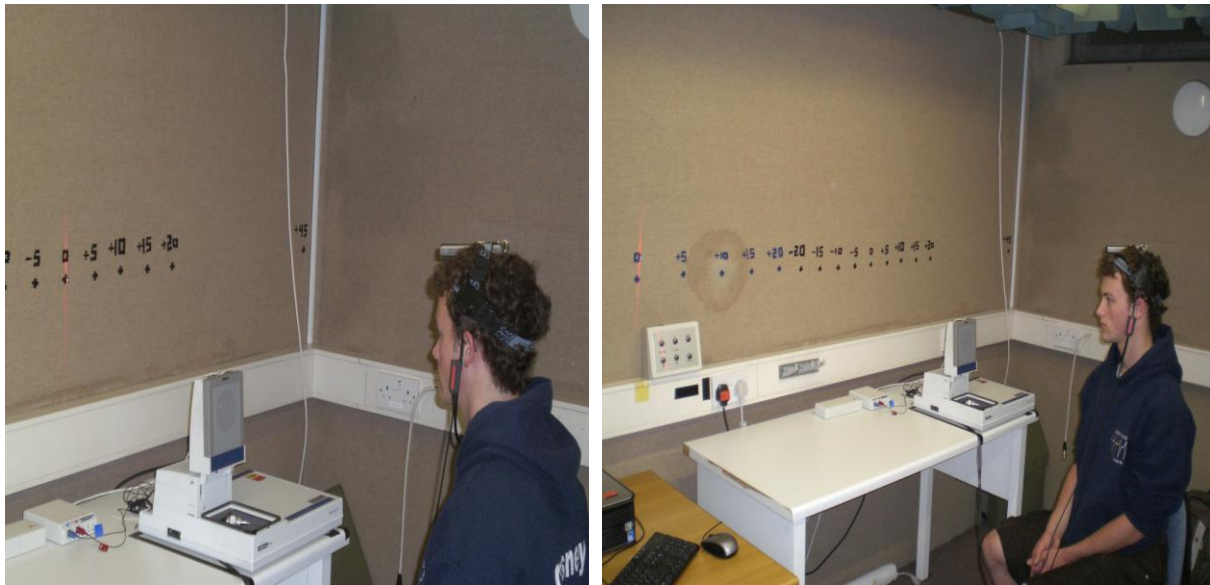
Figure 12: Photograph of the starting or primary head positions for the 0° (left image) and 45° (right image) loudspeaker-to-client azimuth conditions.
