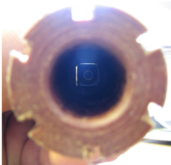
Figure 39 - Photograph looking up the distal end of a stem construct. The stem has been re-inserted by hand following removal prior to \mu -CT scanning. Air gaps are visible indicative of poor interfacial conformity.
