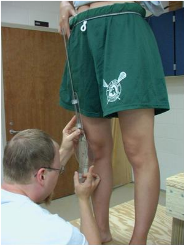
Figure 3.1 – Measuring the Q-angle with participant in relaxed standing, using a Long-arm Goniometer ( www.uncg.edu/kin/anrl/facilities.html ), with permission
