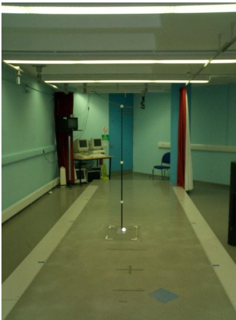
Figure 5.1 – One-metre calibration rod for 2D video motion analysis
