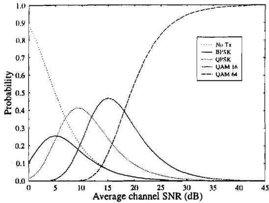
Figure 3: Upper bound probability of the individual modulation schemes for adaptive modulation optimised separately for speech plotted against average channel SNR for a Rayleigh channel
