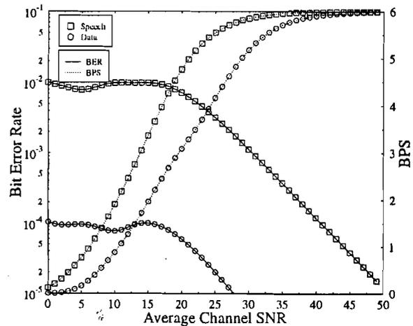
Figure 2: Upper bound BER and BPS performance of adaptive QAM in Rayleigh Channel optimised separately for Speech and Data transfer
