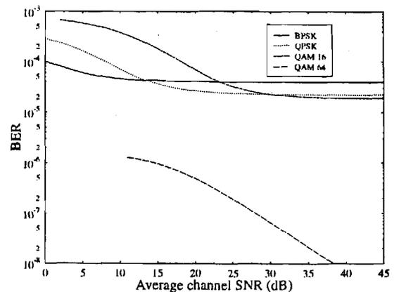
Figure 6: Upper bound BER of the individual modulation schemes for adaptive modulation optimised separately for data transfer plotted against average channel SNR for a Rayleigh channel
