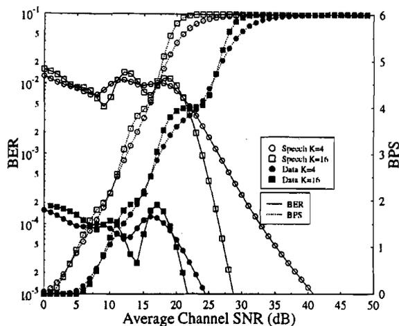
Figure 7: Upper bound BER and BPS performance of adaptive QAM in Rician Channels having been optimised separately for Speech and Data transfer and found by numerical solution
