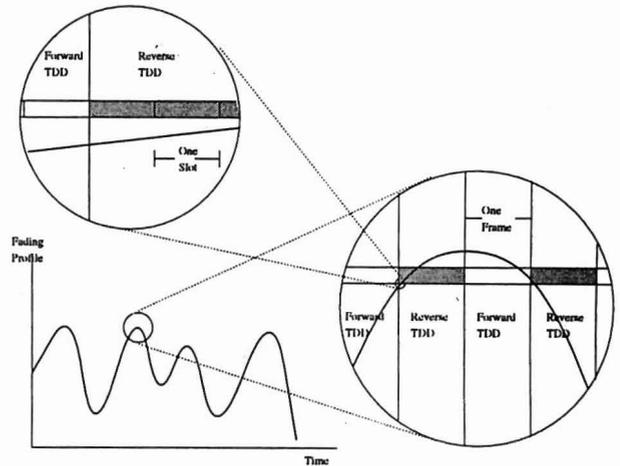
Figure 1: Received power fluctuation over the duration of one TDD slot, when compared with the deviation over the whole channel results in a single slot exhibiting near-Gaussian channel characteristics. The correlation between corresponding slots in adjacent TDD frames may be exploited.
