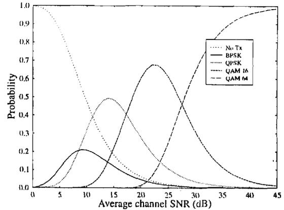
Figure 5: Upper bound probability of the individual modulation schemes for adaptive modulation optimised separately for data transfer plotted against average channel SNR for a Rayleigh channel
