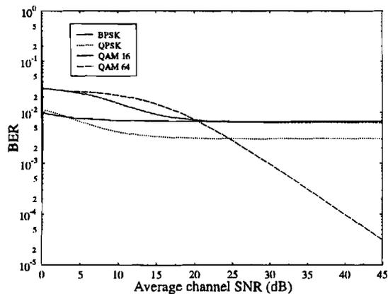
Figure 4: Upper bound BER of the individual modulation schemes for adaptive modulation optimised separately for speech plotted against average channel SNR for a Rayleigh channel
