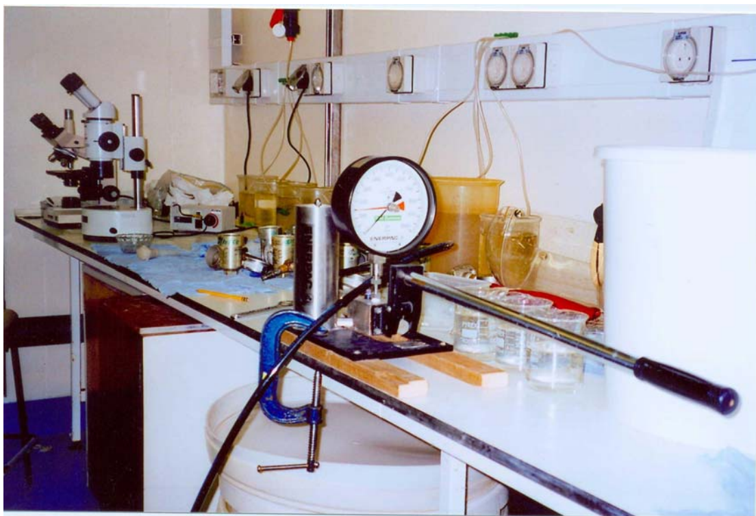
Fig. 3.5. Enerpac hydraulic hand pump used to pressurize the modified chambers using fresh water. (Photograph by Francisco Benitez)
