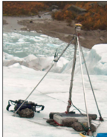
Figure 4. Base Station installation on glacier
