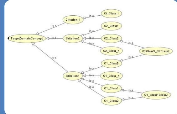
Structure of the View Inheritance ODP for the representation of Fault
