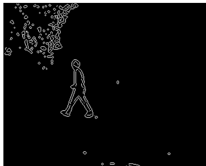
(h) Canny edge-detected image
