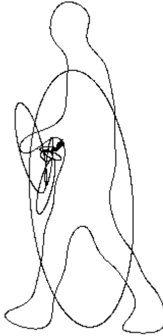
FIGURE 3.3: Example of how a shape is reconstructed from rotating elliptic phasors.
