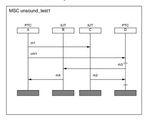
First note that the ordering of events in the PTC is still tightly coupled. With this coordinating message we have forced !m2 to be earlier than !m3. Also it is clear that there is no other way we can force  $!m2 <_T !m3$  to occur, so such a CM is the minimum necessary additional structure we can add.
