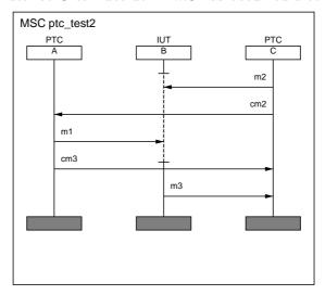
The purpose of cm2 is to force !m1 to be after !m2. The purpose of cm3 is to advise C that A is has sent m1 to the IUT. So long as ?cm3 arrives before ?m3 C can report that the test has passed.
