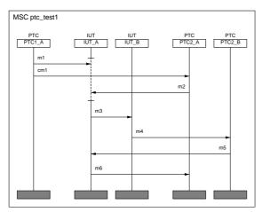
The test to force !m1 to occur after !m2 is constructed analogously.
