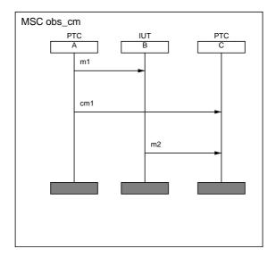
The coordinating message here ensures that the observable ordering is the same as the test ordering, provided that the above latency assumption holds. For the observation ordering to be faithful to the test ordering we have to be able to verify that !m1 < ?m2. If the latency in cm1 is less than the latency in m2 and ?m1 < !m2 then we will have that ?cm1 < ?m2. In this case the only way that ?m2 could be before ?cm1 is if !m2 is before ?m1.
