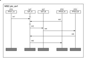
In this example we define PTC1 to consist of the instance PTC1\_A, PTC2 to be instances PTC2\_A and PTC2\_B, and the IUT to be instances IUT\_A and IUT\_B. From now on we assume that any instance which is marked as a PTC is a separate PTC in its own right unless we state otherwise.
