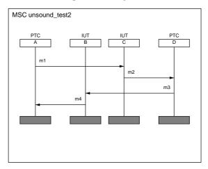
In this case we do not need any coordinating messages to force this order to occur. The test is achieved by PTC D waiting for ?m2 before sending !m3. That is all that is required to enforce the order. In this case the test is sound because we force a send event to wait until a receive event had occurred, in the unsound case we were trying to force a receive event to wait until after a send event.
