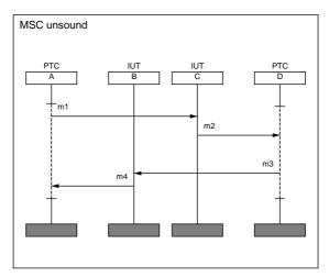
According to the MSC semantics one possible ordering for the PTC events is !m1 then !m3, and then ?m4 and ?m2 in either order. However no matter what coordinating messages we introduce between A and D we can never guarantee that in practise ?m2 occurs after !m3. So no matter how we add coordinating messages the resultant concurrent test will always be unsound.
