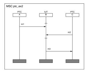
Again two tests are possible, consider the case where we choose to make !m2 occur before !m1. In this case we need one coordinating message to ensure that the send events occur in the correct order and another to ensure that instance C can decide if ?m3 has occurred after !m1.
