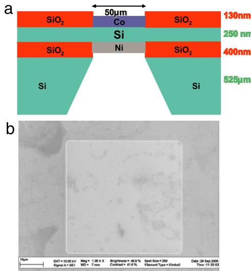
**Fig. 1.** (a) A schematic representation (not to scale) of the vertical Co/Si/Ni back-to-back Schottky barrier based spin injection-extraction device. (b) A scanning electron micrograph of the fabricated device showing the top Co contact.
