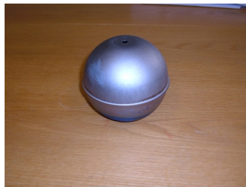
Figure 43: Dry fit assembly of two halves, creating the accumulator
