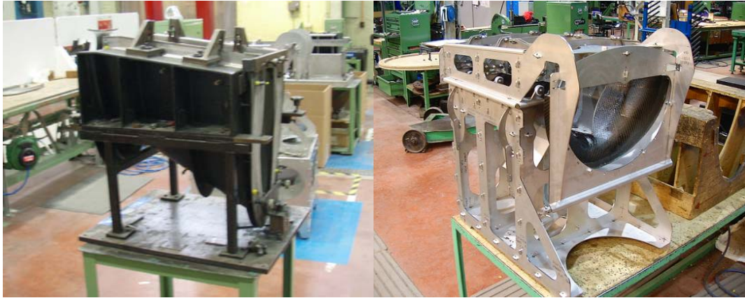
Figure 8: A traditional fixture (a) and the fixture developed by the team in Sheffield (b) for construction and assembly of an engine splitter
