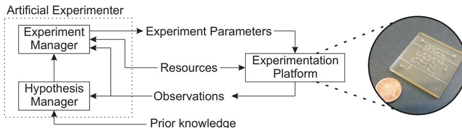
Figure 1. Illustration of a closed-loop autonomous experimentation machine. The artificial experimenter has components to model the data and choose experiments, which are used to provide experiment parameters to the experimentation platform. The experimentation platform then performs the requested experiments, returning the observational measurements as input back to the artificial experimenter. All occurs without human interaction.
