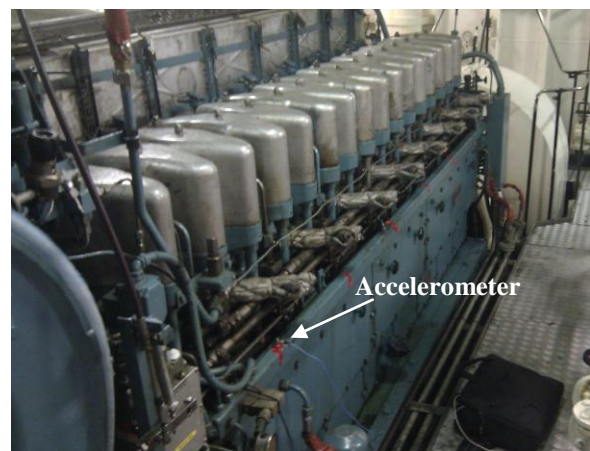
Fig. 2: Eight-cylinder diesel main engine on ferry
