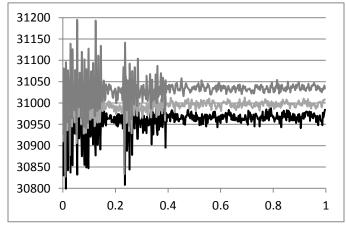
Fig. 2 Example data from a geophone probe showing the different between an event and background noise levels
