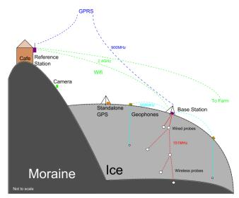
Fig. 1 Schematic of the entire deployment
