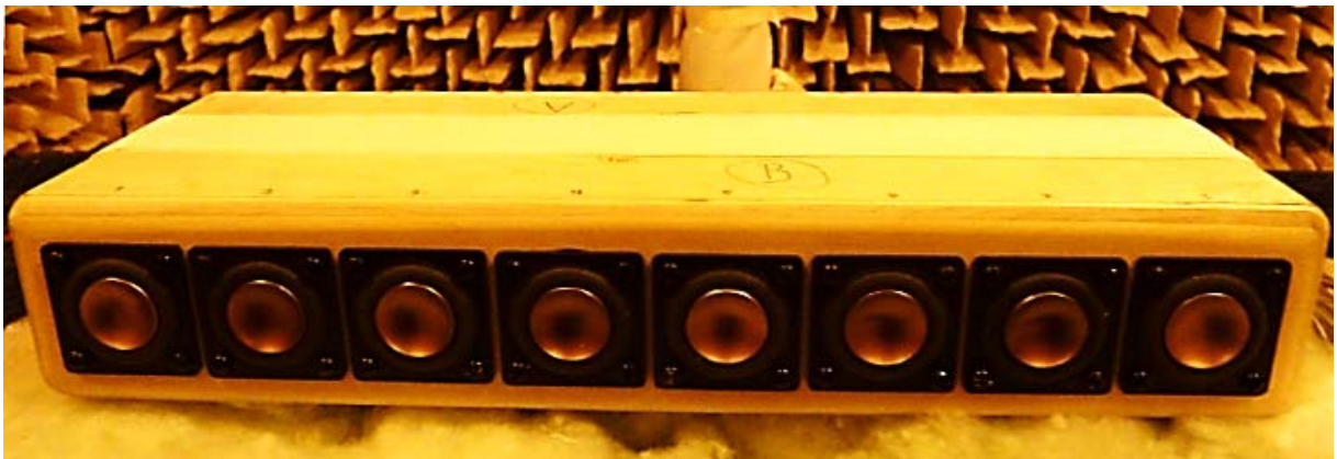
Fig. 2 - Dual-layer loudspeaker array with 16 loudspeakers mounted in an enclosure.
