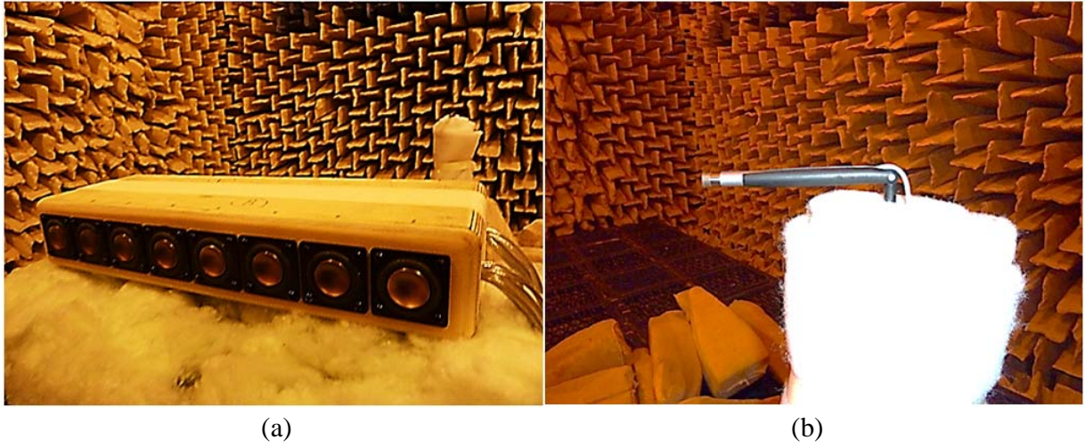
Fig. 7 - Experimental setup for the measurement of the sound radiation pattern: (a) dual-layer loudspeaker array installed on a turntable in the ISVR anechoic chamber and (b) omnidirectional measurement microphone arranged at 1.5 meter away from the loudspeaker array.
