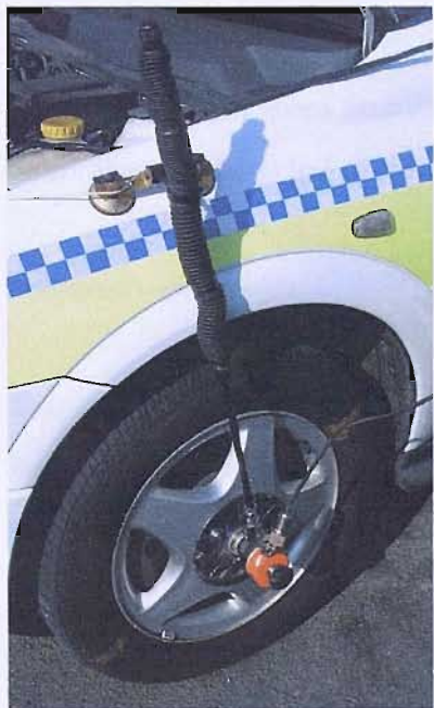
Figure 114 The Datron Corrsys WRT wheel rotation sensor in position
