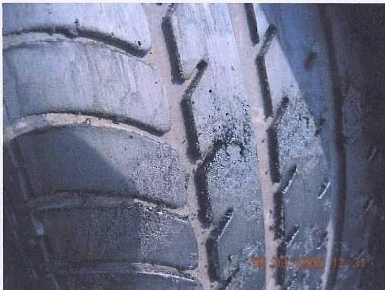
Figure 146 Oily deposit and bitumen observed following NOABS test on SMA in Dorset
