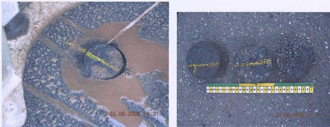
Figure 122 Marked skid orientation and Cored NTS
