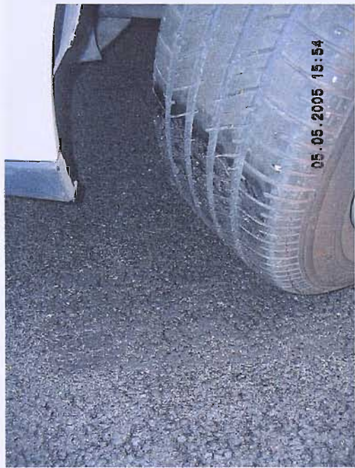
Figure 144 Oily deposit observed following NOABS test In New Zealand
