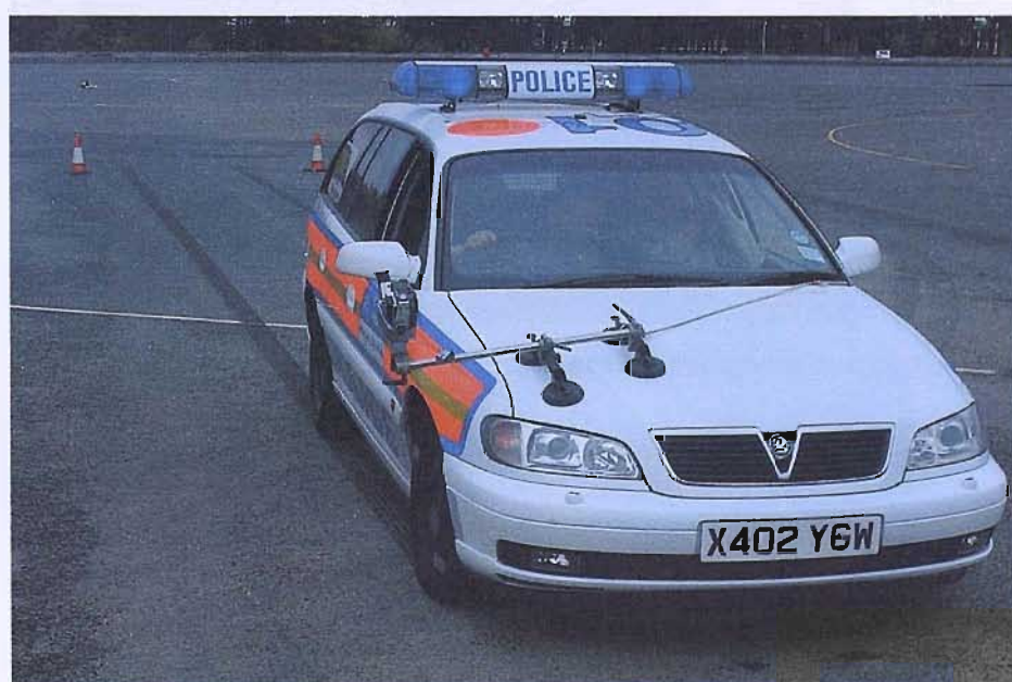
Figure 135 External video camera mounting on skid car
