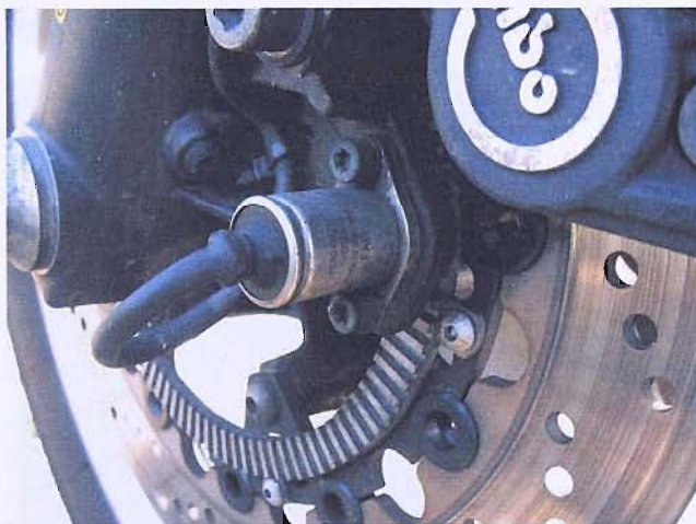
Figure 2 Front ABS sensor of BMW K 1100 LT SE, Bj. 1994 (Source: Wikimedia Commons)
