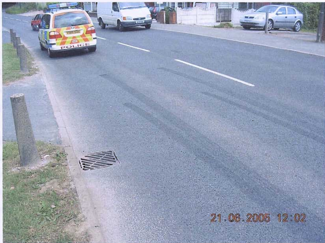
Figure 112 Testing in Derbyshire, NOABS skid marks visible
