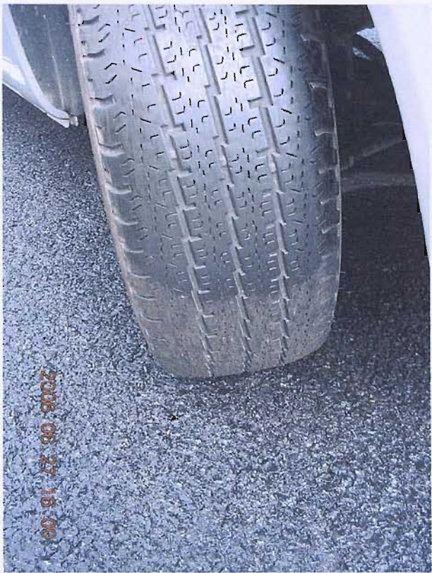
Figure 143 Oily deposit observed following NOABS test at Madingley
