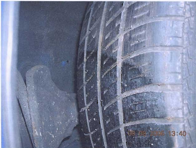
Figure 145 Oily deposit observed following NOABS test on SMA in Devon
