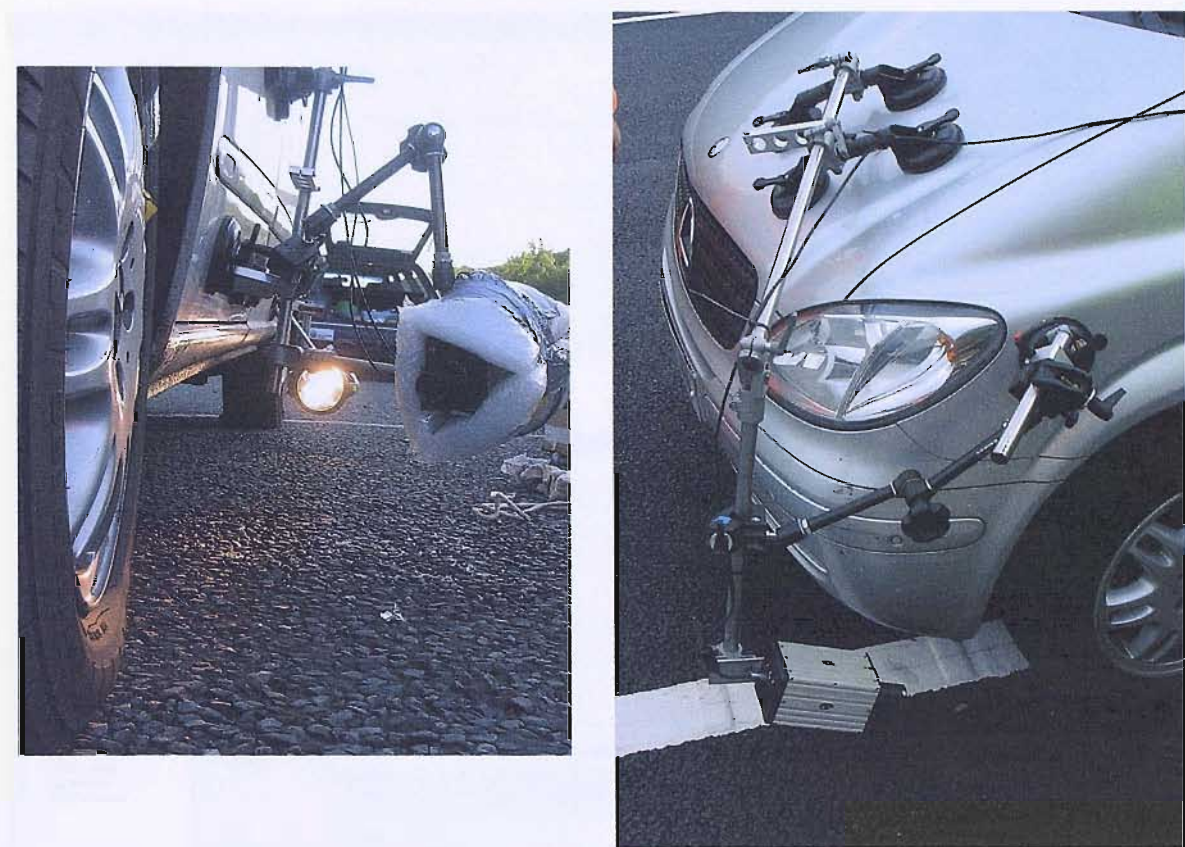
Figure 89 FLIR P65 Camera on Mercedes Vito Van using Manfrotto mountings
