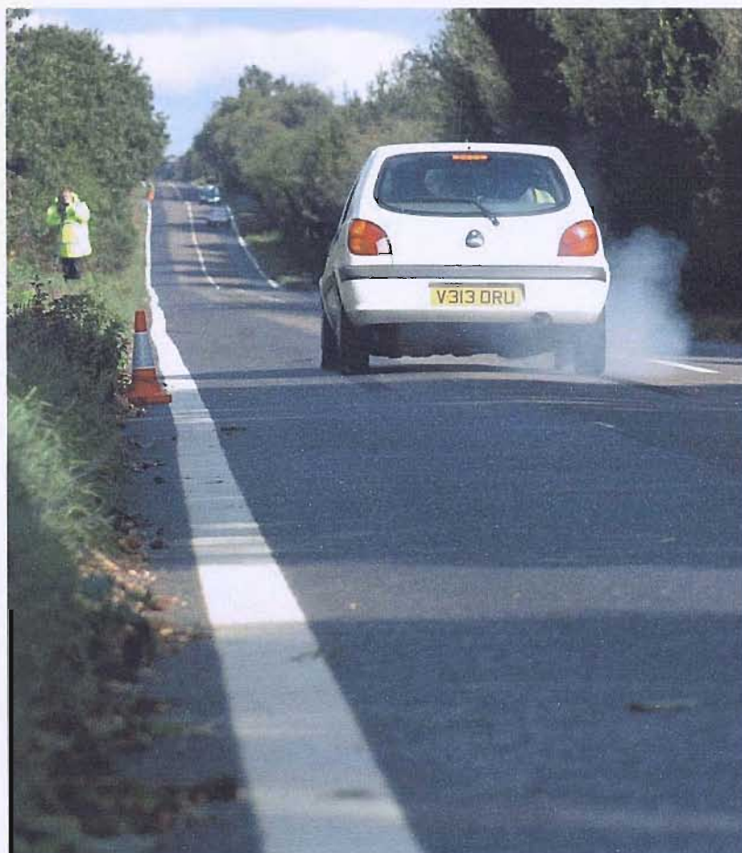
Figure 85 Skid test on split surface (PTS on right NTS on left)
