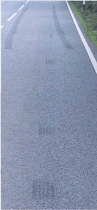
Figure 141 ABS “dashes” observed on an NTS in Dorset following testing
