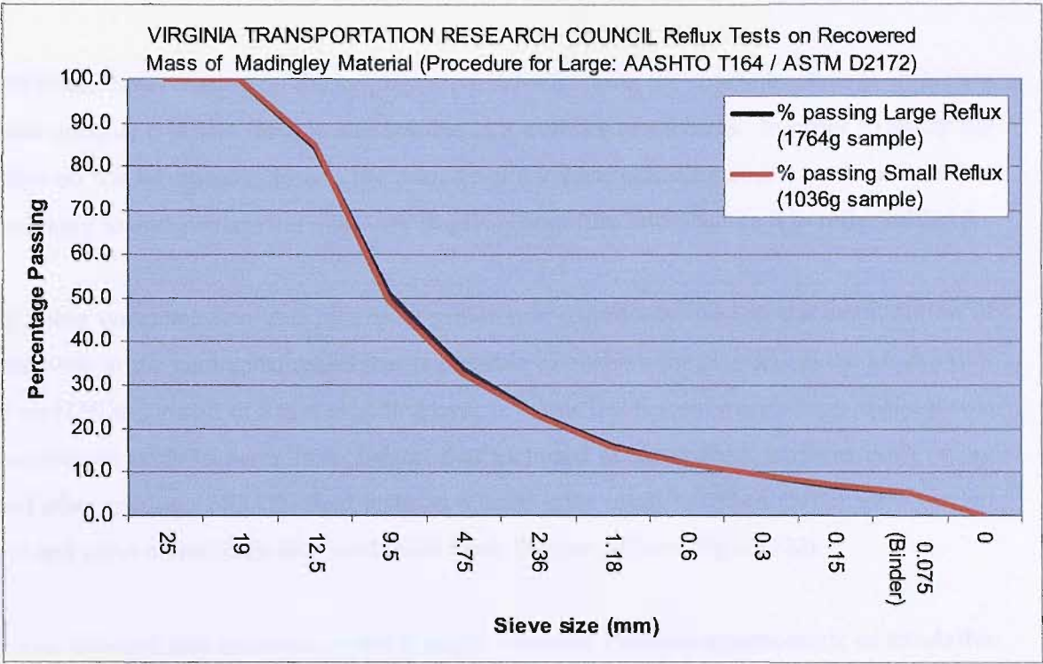
Figure 120 VDOT PSD for the recovered Madingley bituminous materials
