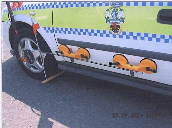
Figure 77: Infra red Sensor Trial Equipment (top left to bottom right) Data recorder, temperature sensor locations (left - tyre, right - road), data recorder and display, wheel speed detector, sensor array mounted using adapted chalk gun mounting (photos by the Researcher)
