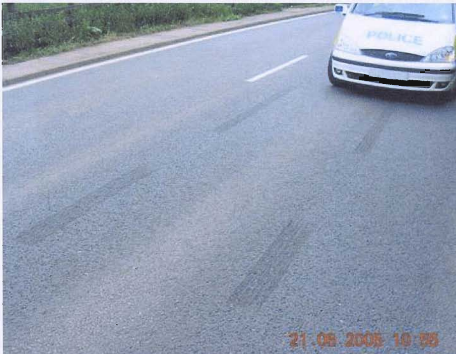
Figure 142 Semi continuous ABS “dashes” observed on an NTS in Derbyshire following testing
