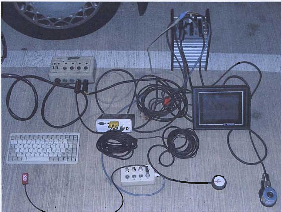
Figure 115 The data logger, GPS and antennae and accelerometer
