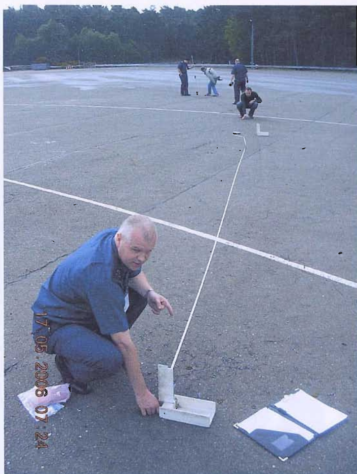
Figure 134 Measurement of Visible Critical Speed Marks
