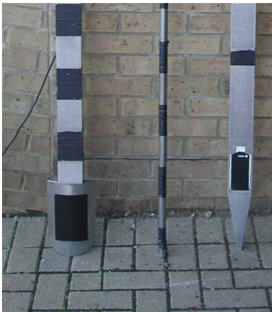
Figure 4.2. Source (left) and Receiver (right) attached to aluminium channels. The measuring pole in centre denotes scale, with each taped section measuring 10 cm long.
