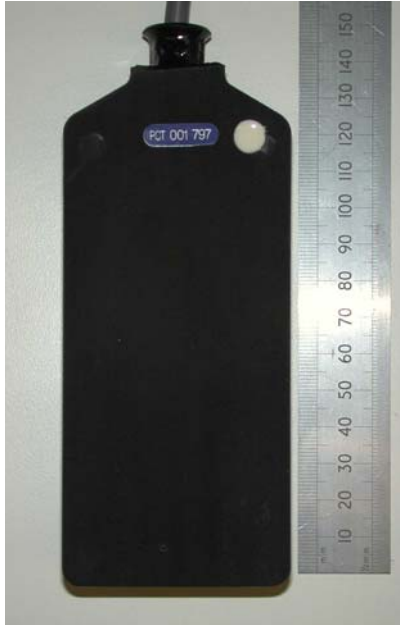
Figure 4.3. Receiver element embedded in polyurethane mould.
