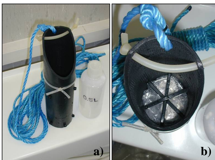
Figure IV.7: a) The "dipper" with a 0.5 L LDPE bottle (18 cm-height); and b) The "dipper" seen from above.
