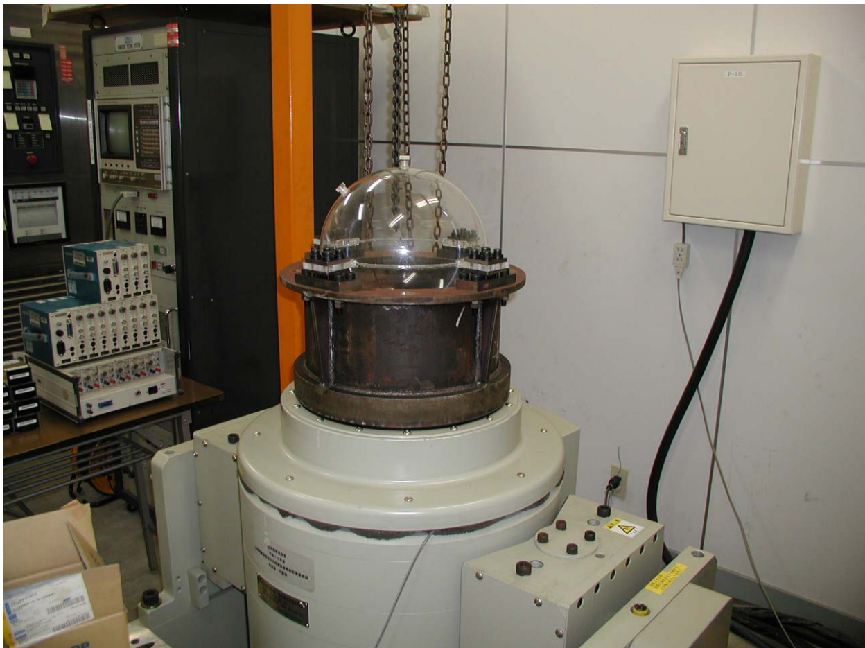
Fig. 1.3 A global view of the tank mounted on the vibration table.
