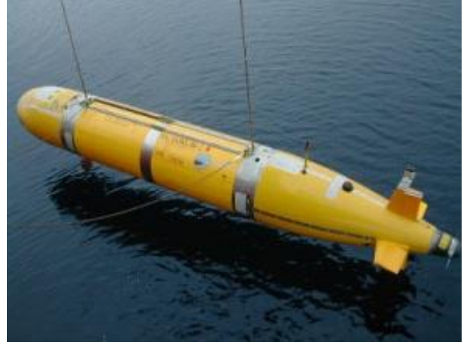
Fig. 1. The AUV Autosub Designed And Developed At The National Oceanography Centre, Southampton.
