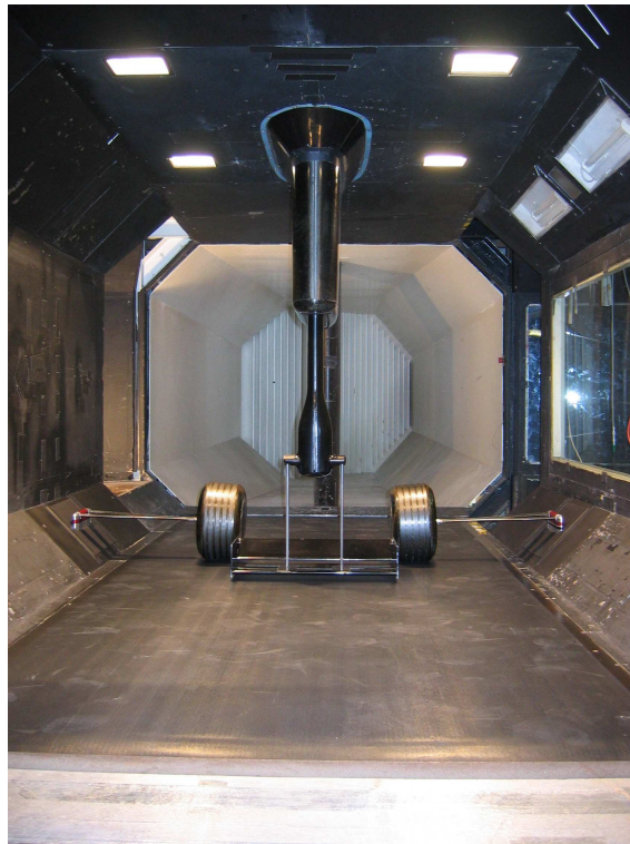
Figure 2.5: Picture of the 7 \times 5 wind tunnel facility with the complete configuration in place, consisting of the force wing model and two 050 dummy wheels.
