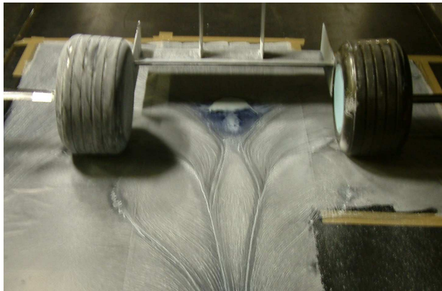
Figure C.7: Picture of oil flow results for the CWW2035 configuration at h/c = 0.211 as a stationary case without ground movement or wheel rotation.
