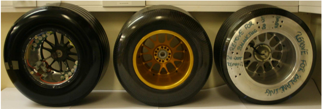
Figure 2.7: Picture showing the three different used wheel models; 020 with McManus pressure system (left), 050 dummy (middle) and 050 with Chell pressure system (right).
