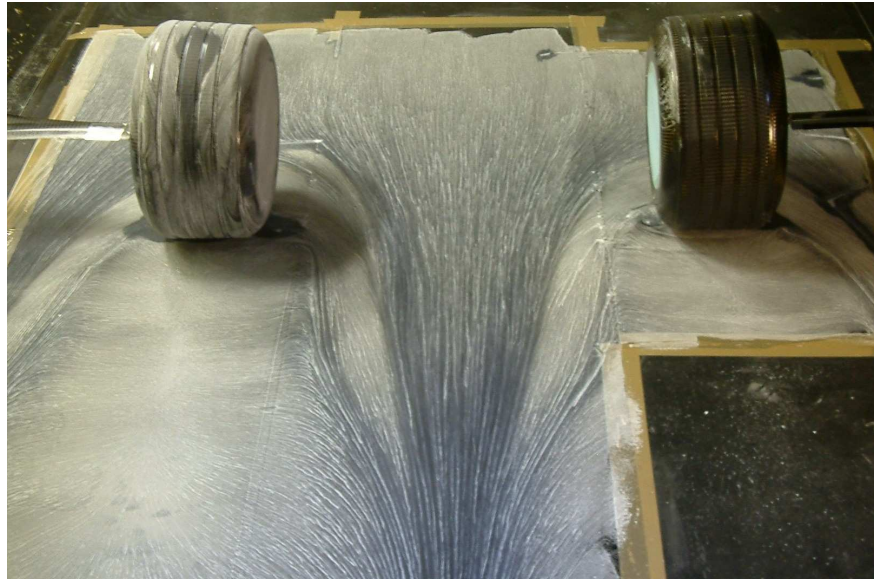
Figure C.6: Picture of oil flow results for the isolated wheel set-up as a stationary case without ground movement or wheel rotation.
