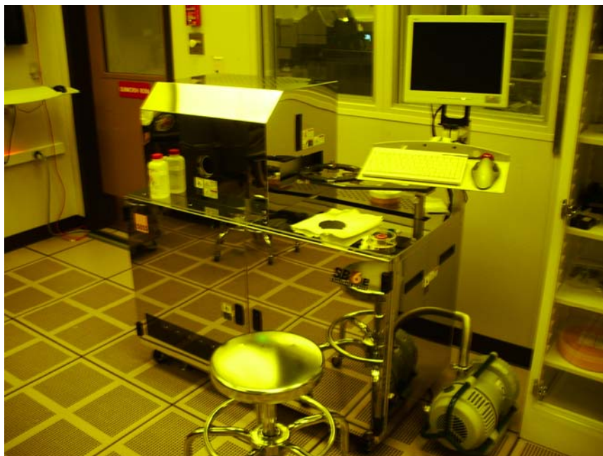
Figure 6.5 Karl Suss SB6e bonder in MNF at the University of Michigan.
