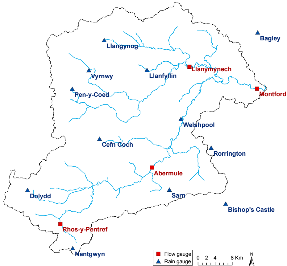
Figure 6.6 Location of precipitation and flow gauges used for hydrological modelling and calibration
