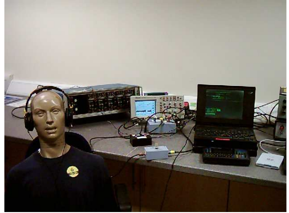
Figure 3.3 Equipment employed to calibrate the acoustic stimuli used in the static experiment.
