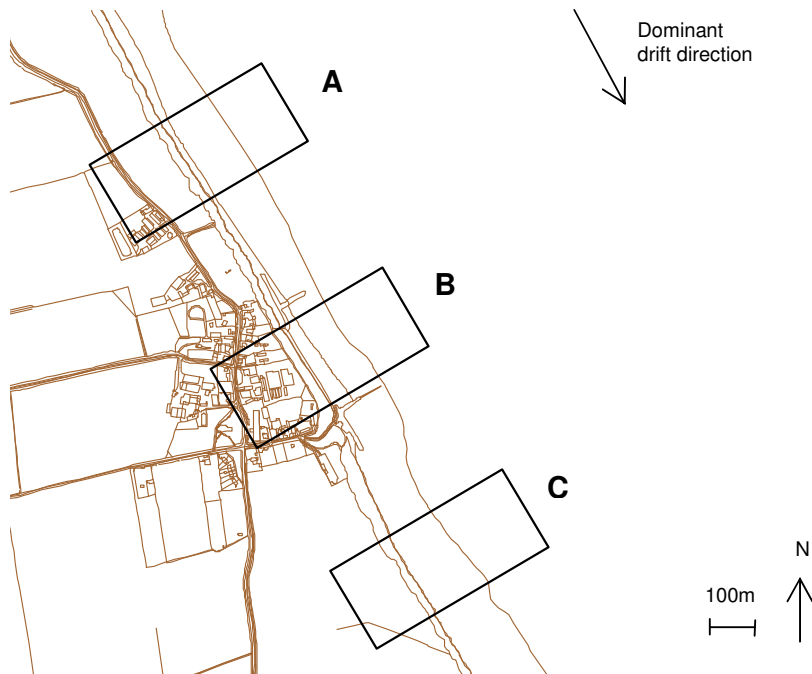
Figure 4.28a – Position of average retreat profiles at Mappleton. Profiles are 200m wide. Profile B is situated in the middle of the defence, and Profiles A and C are located 200m up-drift and down-drift of the defence.
