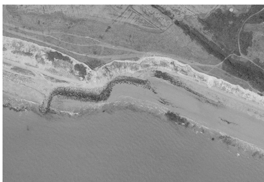
Figure 6.5 (ii) – Four of eight photographs (Panels e-h) showing outflanking and the growth of a crenulate shaped embayment down-drift of Barton-on-Sea from 1967 to 2005 (Aerial photographs from New Forest District Council and the Channel Coastal Observatory, Southampton, see Table 3.5).
