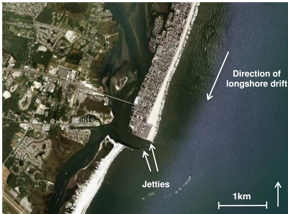
Figure 2.11 - Ocean City Inlet, Maryland. The inlet was stabilised in 1934-1935 and since then, the down-drift coast has been set back over 600m. Erosion increased from 0.6m/yr before jetty construction to 9.3m/yr after jetty construction (photograph from Google Earth, 2007).
