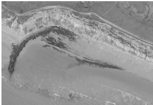
Figure 6.6 (ii) – Four of eight photographs (panels e-h) showing outflanking and the growth of a crenulate shaped embayment down-drift of Becton from 1967 to 2005 (Aerial photographs from New Forest District Council and the Channel Coastal Observatory, Southampton, see Table 3.5).
