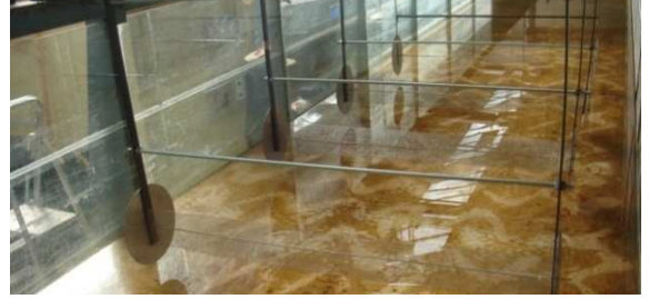
(b) Front view showing end discs to minimize vortices shed from ends.
