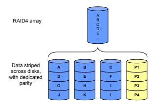
The data is broken down into strips and distributed across all but one of the member disks. The remaining one being the parity, which is the XOR of the data strips. In the layout shown above, P1 is the XOR of A, B and C; P2 is the XOR of D, E and F; and so on.
