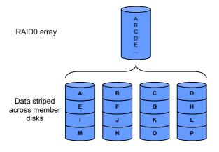
In a RAID0 array the data is broken down into small pieces, called strips, which are then distributed across the member disks
