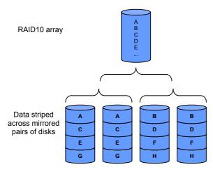
It is suitable for similar applications to RAID1, where data reliability and fault tolerance are more important than cost. An additional benefit of RAID10 over RAID1 is increased performance.
