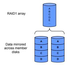
RAID1 provides full fault tolerance for a single drive failure and detected read errors, as a complete copy of the data is available on the mirror disk.
