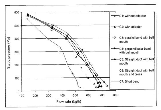
Figure 13 – Static pressure as a function of the flow rate
