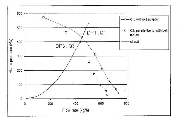
Figure 32 - aerodynamic characteristics for configurations 1 and 3
