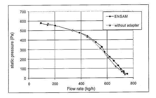
Figure 12 - static pressure measured by the ENSAM, and with the configuration 1 (without adapter)
