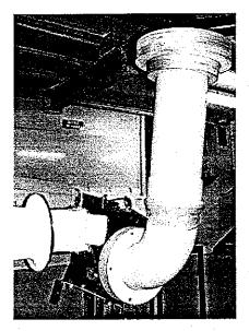
Figure 9 - configuration 4: perpendicular bend with a bell mouth
