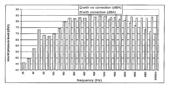
Figure 24 - third octave bands of sound pressure level for the straight duct (Qm=651kg/h) in dB(A)
