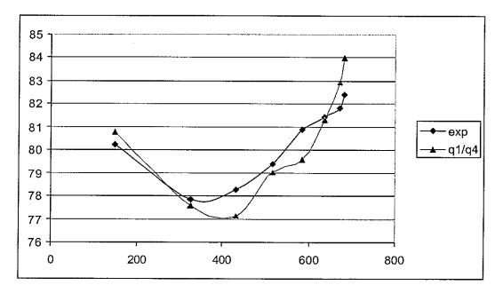
Figure 35 - Sound power in dB(A) for the configuration 4
