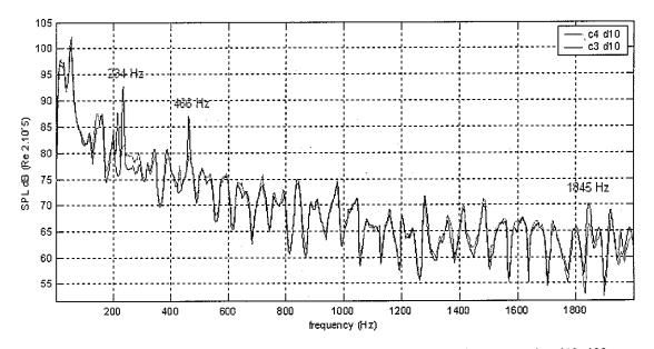
Figure 29 - SPL Spectra for the configurations 3 and 4 at the same diaphragm opening d10=180mm
