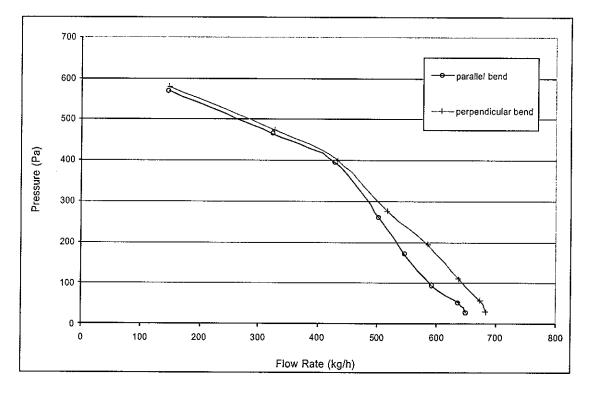
Figure 14- Static pressure with the parallel and perpendicular bends
