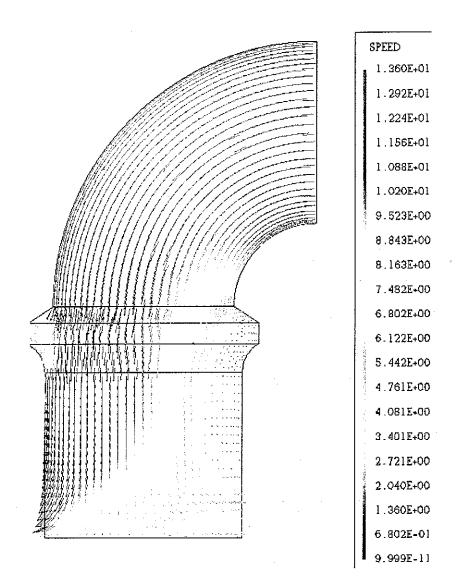
Figure 15 - repartition of the velocity field inside the wheel after a bend
