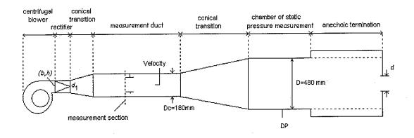
Figure 1 – Scheme of the fan rig
