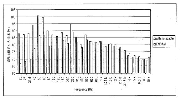
Figure 26 – Third octave spectra for the ENSAM/without adapter configurations (Qm=550 kg/h).No corrective factor C applied.
