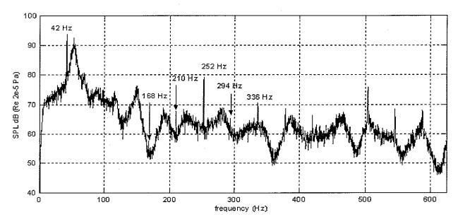
Figure 20 - Multiple pure tones (configuration 2, Qm=439 kg/h)
