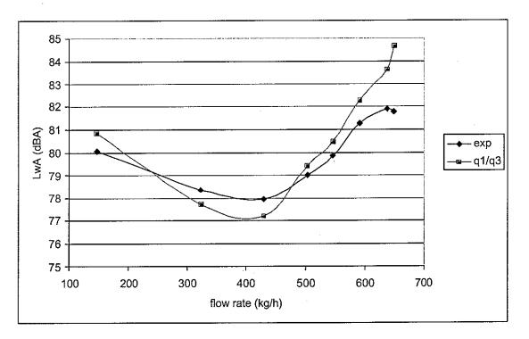
Figure 34 - Sound power in dB(A) for the configuration 3
