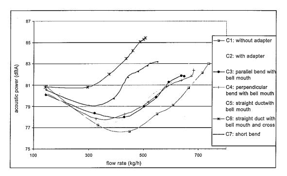
Figure 17 - Sound power level in dB(A)
