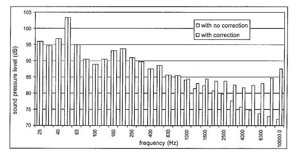
Figure 25 - third octave bands of sound pressure level for the straight duct (Qm=651kg/h) in dB
