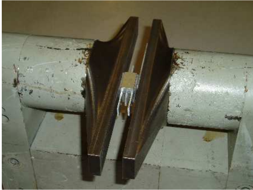
Figure 4.4: Curing specimen placed between two magnetic guiders attached permanent magnet to get magnetization effect
