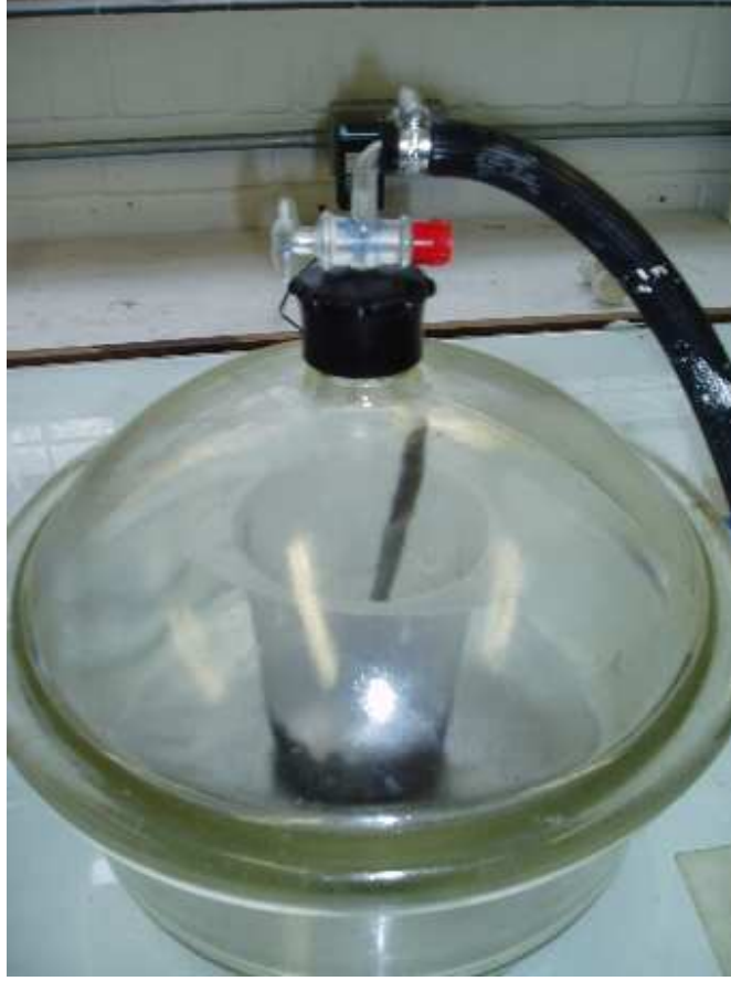
Figure 4.2: Degassing with vacuuming chamber
