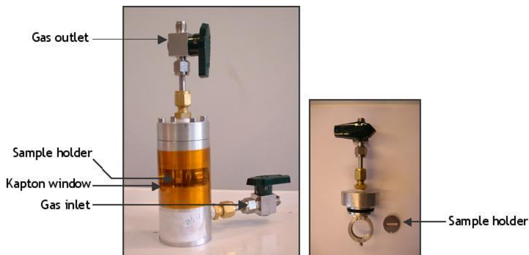
Figure 2- 12 EXAFS gas treatment cell.
