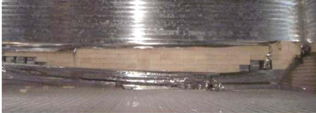
Figure 2.1: Severe damage to a membrane LNG containment system due to sloshing at a low filling level (from vom Baur, 2009). The primary barrier is detached and the primary insulation is visible. In some locations primary insulation boxes are missing and the secondary barrier can be observed
