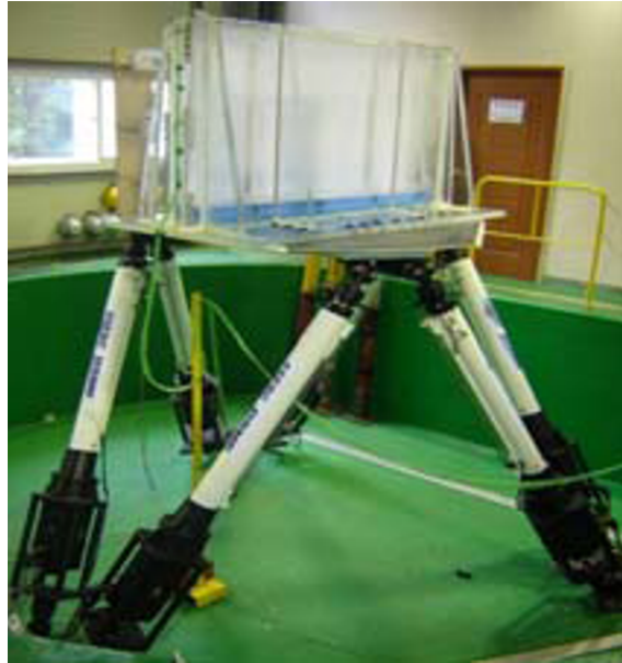
Figure 2.9: 6 DOF sloshing rig used for LNG carrier design with hydraulic actuators (from Jeon et al. , 2008). Costs including instrumentation can approach £250,000.
