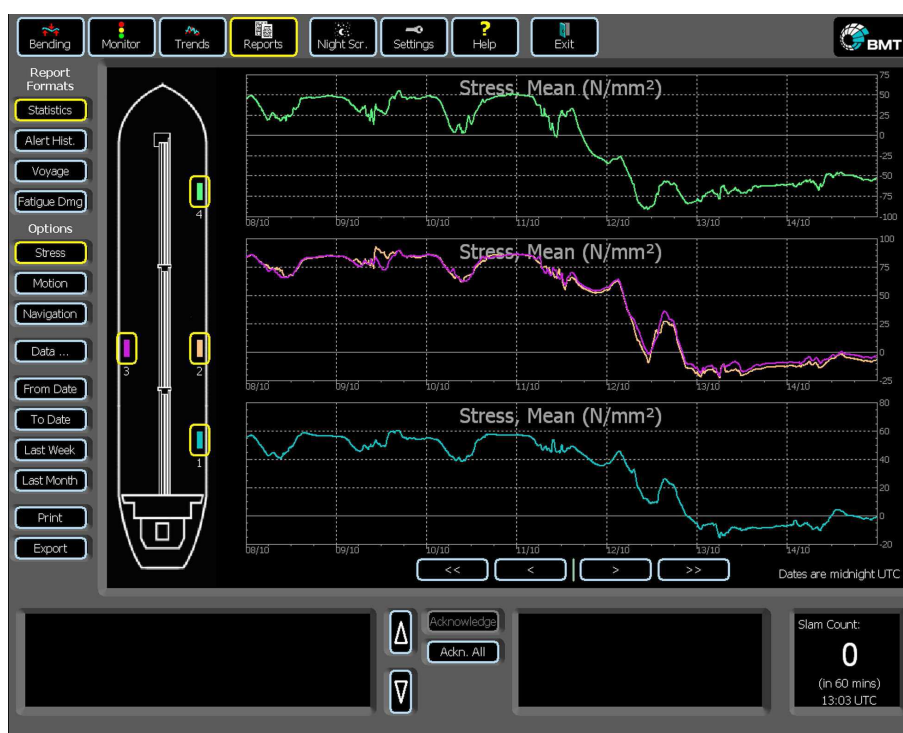
Figure 1 - Typical Display from BMT SeaTech's Hull Stress Monitoring System
