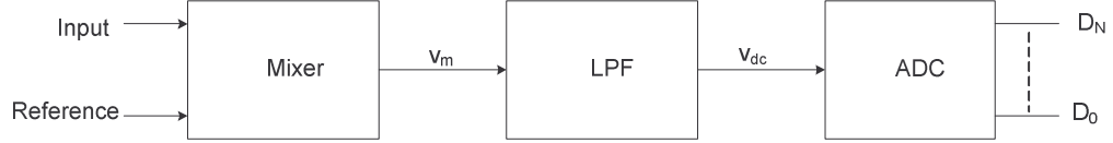
Figure 5-5: Proposed Time Measurement Architecture
