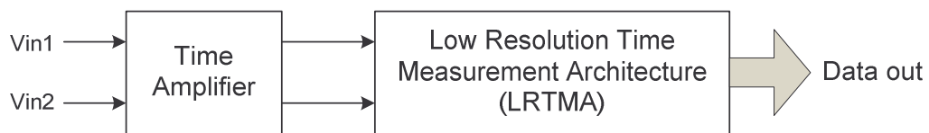
Figure 5-2: Low resolution time measurement architecture (LRTMA) with time amplifier
