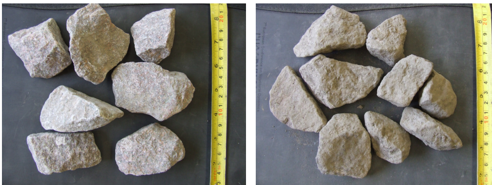
Figure 4.5. Photographs of samples of the new ballast, left-hand pane, and old ballast, right-hand pane.
