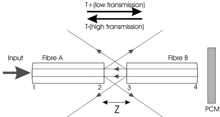
Fig. 5. Schematic of two fibre geometry separated by distance  $z$ , showing directions of low ( $T(+)$ ) and high ( $T(-)$ ) transmission. PCM: phase conjugate mirror.
