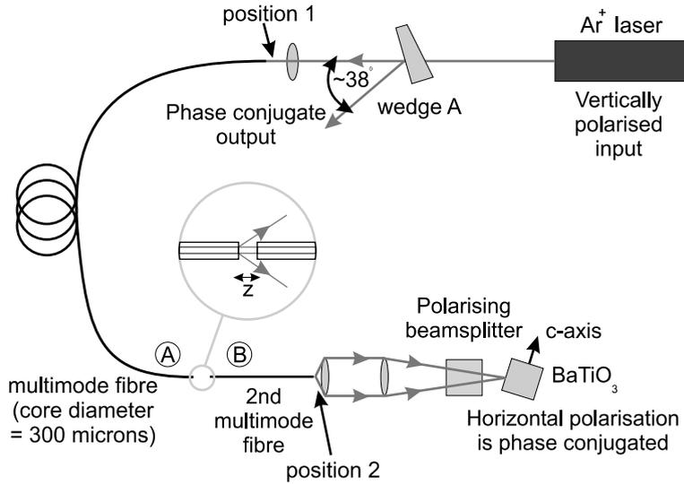
Fig. 4. Use of two separate multimode fibres to allow variation of modal content for subsequent phase conjugation.
