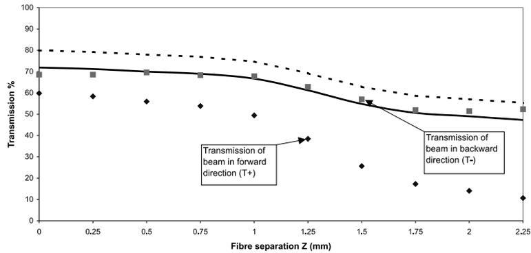
Fig. 6. Measured values for  $T(+)$  and  $T(-)$  as a function of separation,  $z$ .
