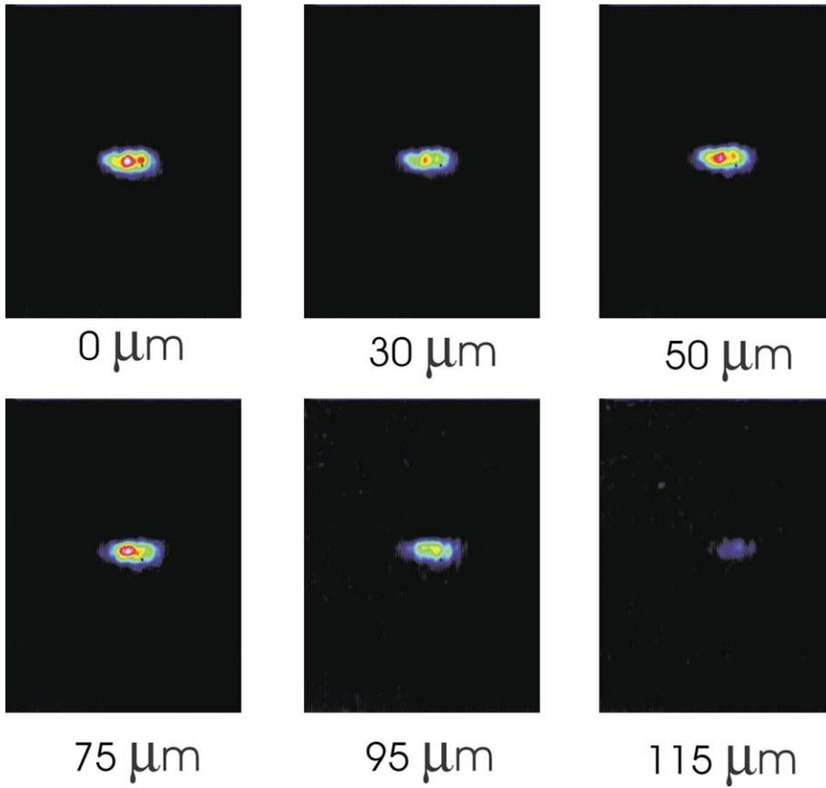
Fig. 7. Phase conjugate output for lateral misalignment between the two fibres.
