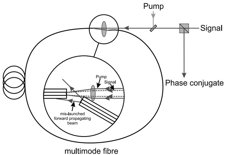
Fig. 8. Schematic showing implementation of NRTE in gain-grating fibre resonator geometry.
