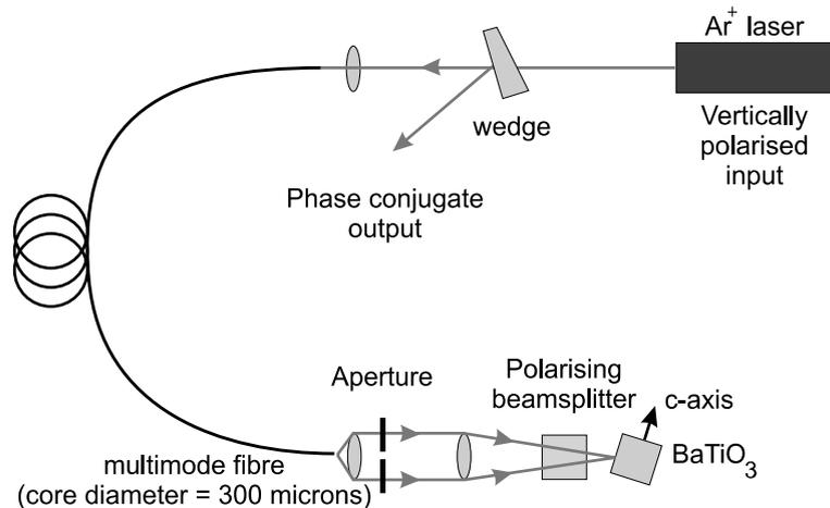
Fig. 1. Schematic of set-up used to investigate phase conjugate correction of modal distortion in a passive multimode fibre.
