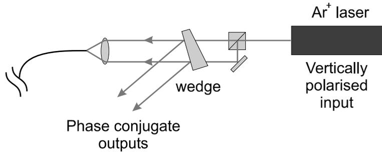
Fig. 3. Modification to Fig. 1 to allow two simultaneous input beams.
