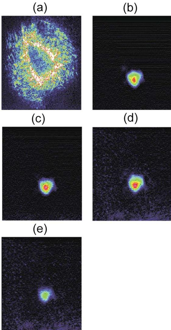
Fig. 2. Spatial output from the multimode fibre: (a) the single-pass output at the end of the fibre; (b–e) the phase conjugate output recorded at the input end of the fibre after double pass and modal correction after passing through an on-axis aperture of diameter 7 mm (b), 3 mm (c) and 2 mm (d); (e) the phase conjugate after passing through an aperture of diameter 3 mm, centred 2 mm off-axis.
