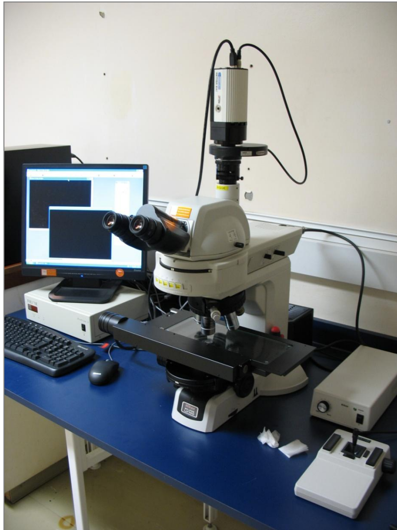
Figure 3: EDIC microscope with attached camera and computer system.
