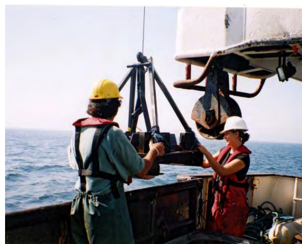
Figure 4.2: Deployment of a typical 0.1 m 2 mini-Hamon grab.
