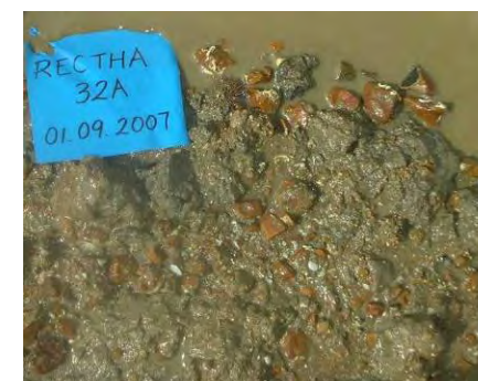
Figure 4.23: Muddy sandy gravel typical of infaunal assemblage B1 (survey site 32).
