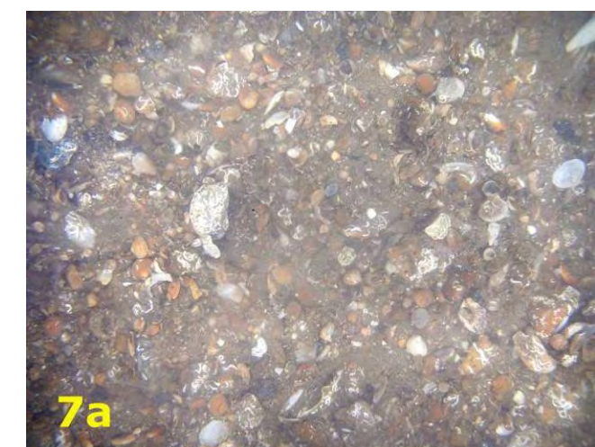
Figure 2.14: Sandy flint and shell gravel seabed from a trough between the sandbanks in the Western Zone (grab sample location 7).
