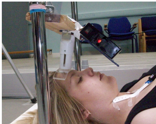
Figure 6.4 Head raise position exceeding the 1.0 – 1.25 cm range
