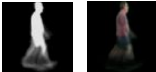
(e) The masks are averaged across a single gait cycle to create the Average Silhouette Signature (f) The colour silhouettes are averaged across a single gait cycle to create the Average Colour Silhouette Signature
