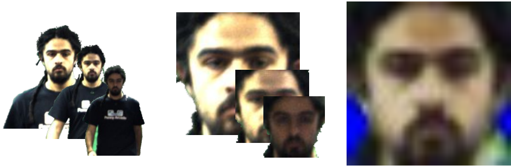
(c) The connected region is isolated by using as the largest connected region above as a mask on the original frame (d) The Viola-Jones faces detector implemented in the OpenCV library is used to locate the face in the isolated region (e) Each face is normalised to 32x32 coloured image. A single average face is generated and used as the signature
