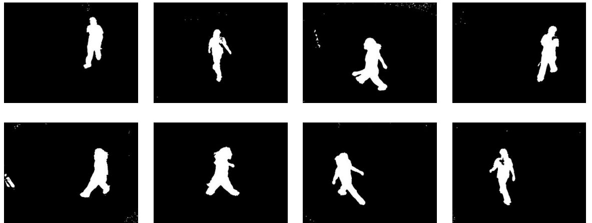
(b) Each camera is background subtracted. The largest connected area is the subject's silhouette
