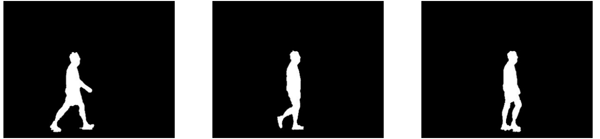
(b) Each frame of a given gait cycle walk has the background subtracted. The subject is the largest connected region
