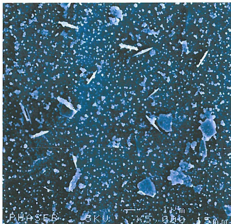
FIGURE 3.14: SEM micrograph of 'phase B' crystals (needle-shaped) in devitrified 71Ga_2S_3:29La_2S_3 glass.
