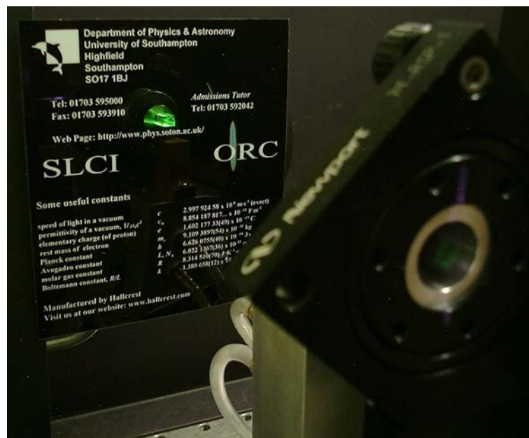
Figure 3-13: Picture of Er:YAG LMA PW laser output, viewed on a heat sensitive card.
