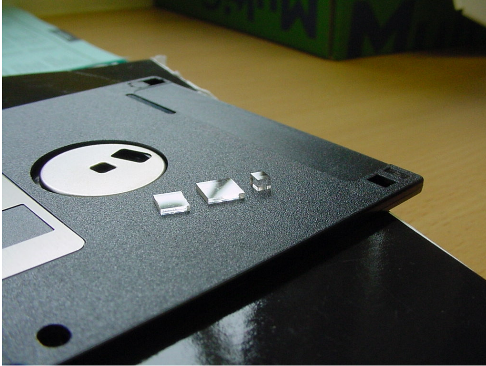
Figure 3.12: A photograph of three direct-bonded \text{LiNbO}_3 planar waveguide devices. The sample to the left is the PPLN device described in this chapter.
