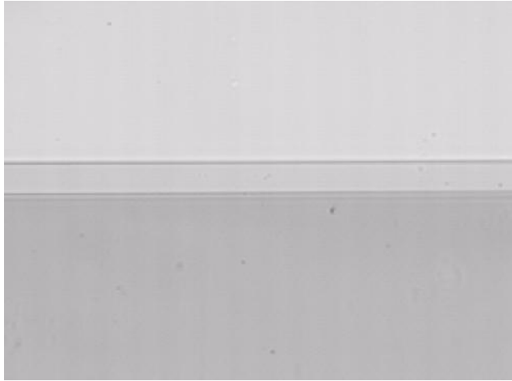
Figure 3.14: A photograph of the polished end-face of a 12\mu\text{m} thick PPLN waveguide (running horizontally through the middle of the picture) buried in \text{LiTaO}_3 by direct bonding and precision polishing techniques. Taken at 50\times magnification, this picture demonstrates the uniformity of each direct-bonded interface.
