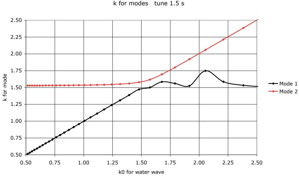
Figure 1: Wave numbers for modes 1 and 2 vs  $k_0$ , for  $k_b = 1.50$
