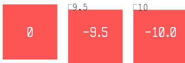
Figure 5-21 Design of vertical alignment tolerance features that, in these features, are -9.5 and 10 \mu\text{m} below the plain of the ideal alignment pattern (zero).
