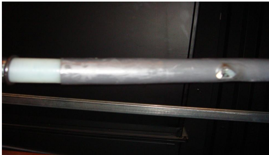
Figure 9-7: Rejoined degassed cable's self bonding wrap meltdown
