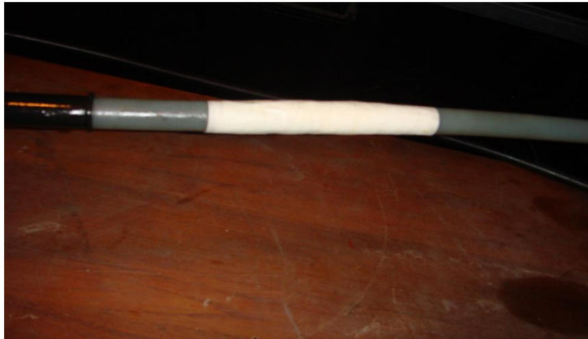
Figure 9-8: Illustration of a rejoined degassed cable under fibreglass wrap
