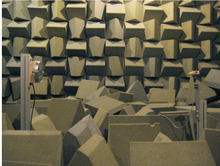
Figure 4.14: Measurement set-up in the anechoic chamber (ISVR). The floor of the chamber is covered with the sound absorbing materials.
