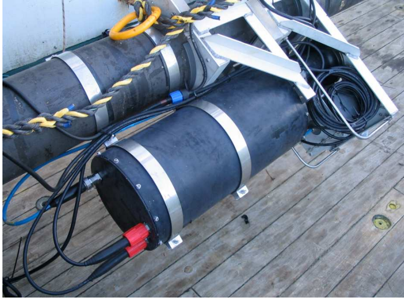
Figure 4.7: The pressure housing as mounted on the buoy.
