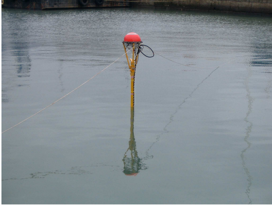
Figure 5.7: The buoy in the docks at the National Oceanography Centre, Southampton, as part of a calibration test.
