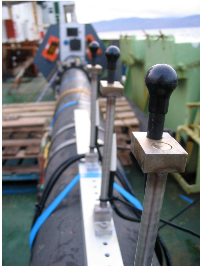
Figure 4.10: The three hydrophones used on D313. The photograph looks down the buoy towards the base, and the transmit transducers are visible in the background. Hydrophone separation is 0.2 m and the distance from the hydrophone furthest from view to the transmit transducers is 3.86 m.
