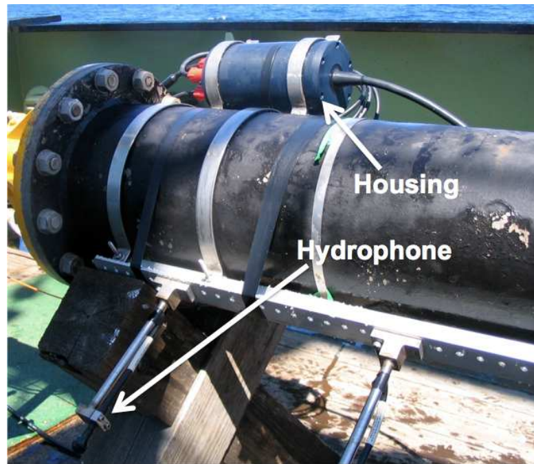
Figure 4.6: The pre-amplifier housing mounted just behind the hydrophones. One of the hydrophones, mounted on the protruding arm, can be seen in the bottom left of the photo.
